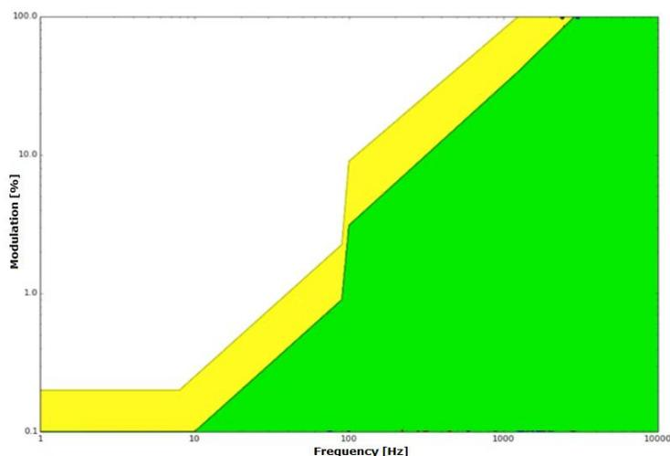
Thanks to the 4kHz dimming frequency the MINI-1CV allows to reduce the Flicker phenomenon.
